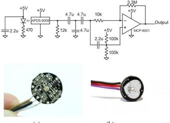
(a) (b) FIG5.2.1 SO00837PS sensor (a)Back side (b) front side
