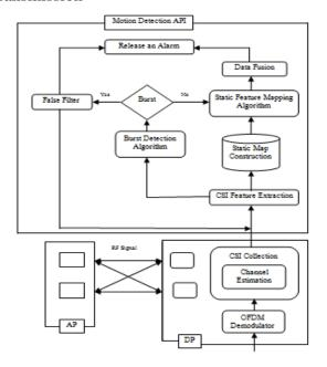
Fig. 1: System Architecture
