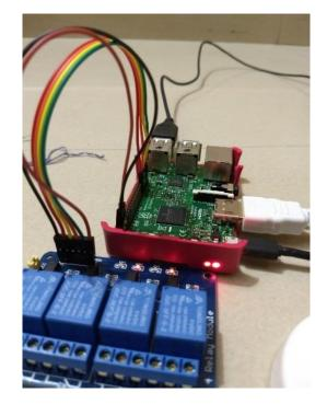
Fig. 7 Relay connected with Raspberry pi
