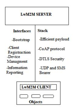
Figure 1: Architecture of LwM2M Enabler
