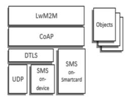
Figure 2: The protocol stack for LwM2M Enabler.
