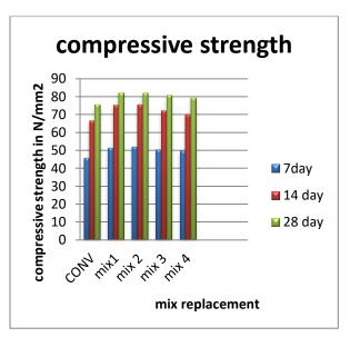
Fig 1show compressive strength of concrete
