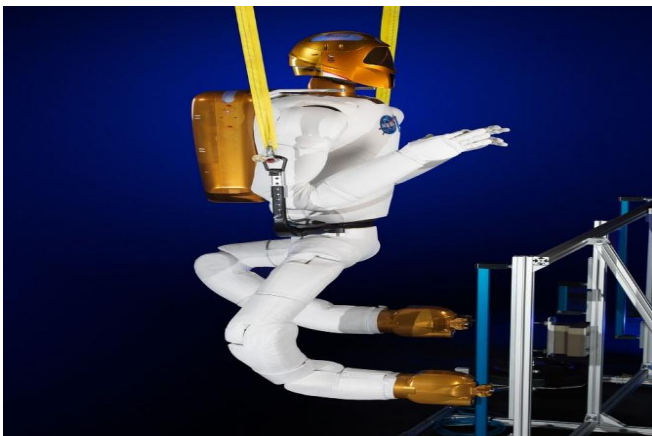
FIG 2: R2 with new Climbing Legs
